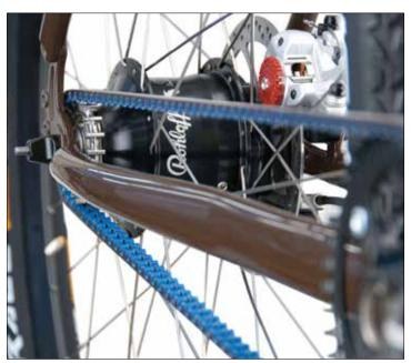
The Divide's drivetrain with Rohloff Speedplay hub and Gates Carbon drive.
